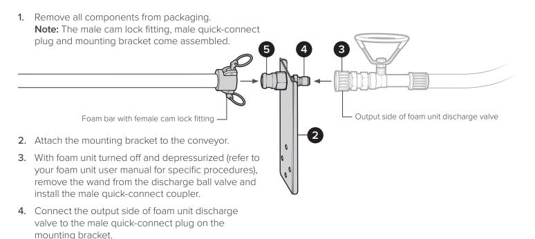
5. Connect foam bar to the male cam lock fitting.
