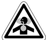
Mixing an alkaline with an acid may result in a chemical reaction. Overheating of mixture may cause it to splatter caustic compounds or release hazardous fumes, gas and vapors. Always flush the unit with fresh water thoroughly when switching from an alkaline to an acid or an acid to an alkaline.
